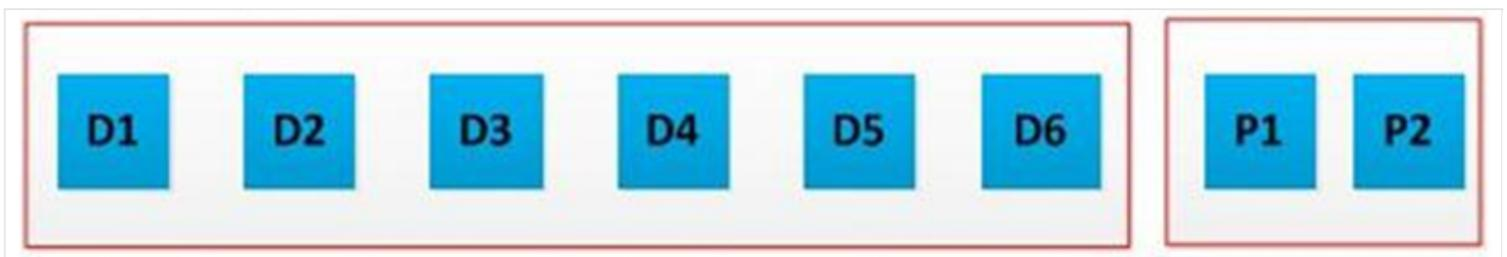
6 data blocks generate 2 CRC blocks, and the data blocks are recoverable if up to 2 blocks are lost. (This is configurable.)
