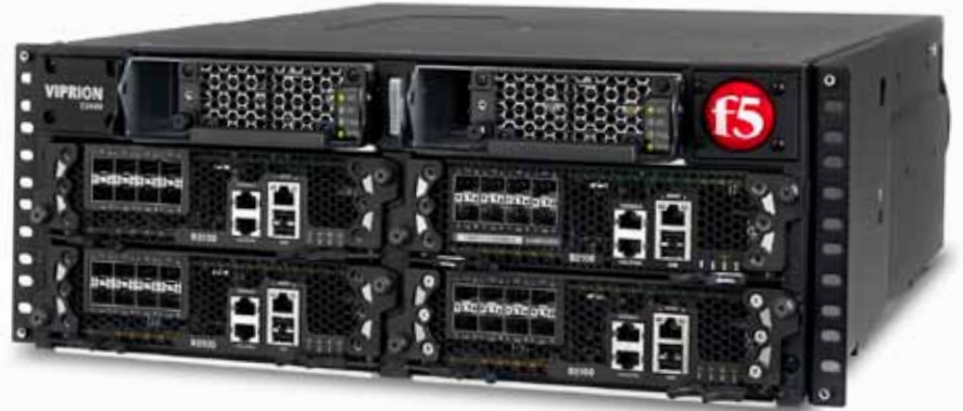
Figure 6. The VIPRION* 2400 chassis supports up to four Intel® Xeon® processor-based blades.
