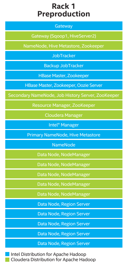
Figure 3. The preproduction environment enabled us to validate our processes. This environment was powered by 128 cores (using Intel® Xeon® processors) and eight data nodes populated with actual data volumes.
